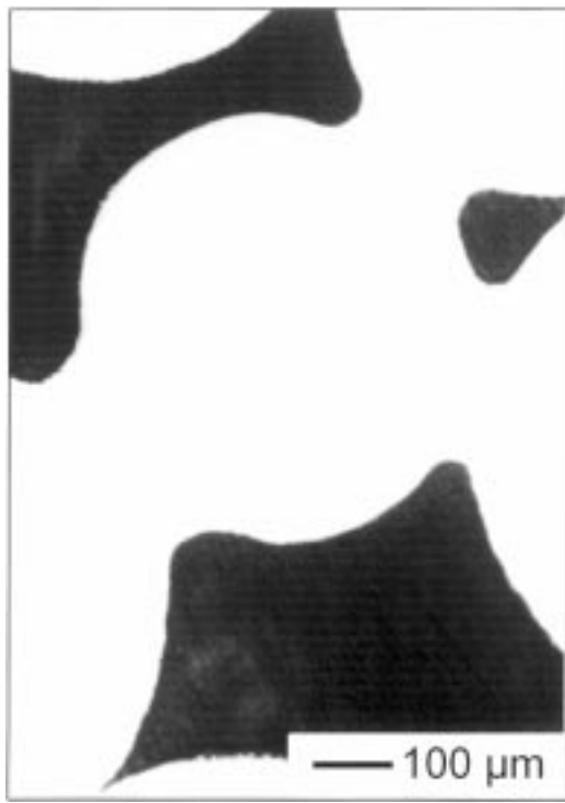
Figure 2 Sinter neck geometry of a non-graded specimen achieved by the addition of 1.5 wt % Si to spherical Ti particles (500/700 μm; milled; 1510 °C, 1 h; cross-sectioned; light-microscopy).
